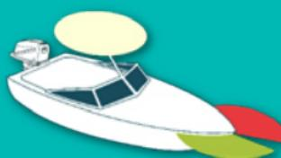
When underway, powerboats less than 12 metres long may combine their stern and masthead lights into a single all-round white masthead light. The boat should also have red and green sidelights.
