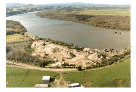
Figure 2: Extraction processes and material stockpiles are common sources of wind-blown dust
