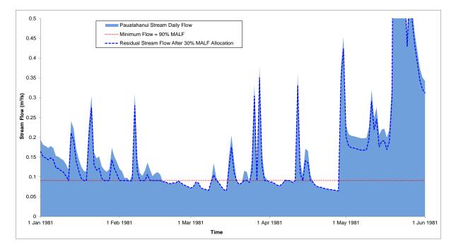
Figure 3. Hydrograph of Pauatahanui Stream showing the natural and residual flows
