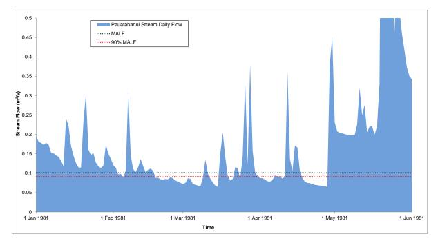
Figure 2. Hydrograph for the Pauatahanui Stream in a drier than average year (1981)
