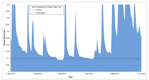
Figure 1. Hydrograph for the Pauatahanui Stream in a moderate year (2014)
