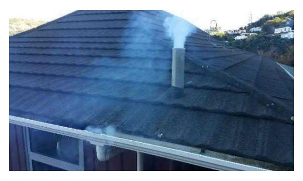
Figure 10. Smoke testing indicating presence of stomwater connections to the wastewater network. Image courtesy of Wellington Water (<a href="https://www.wellingtonwater.co.nz/faqs/wastewater/smoke-testing/">https://www.wellingtonwater.co.nz/faqs/wastewater/smoke-testing/</a>)
