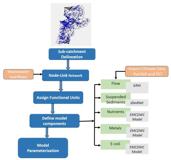
Figure 2.1: Porirua catchment conceptual Source modelling framework
