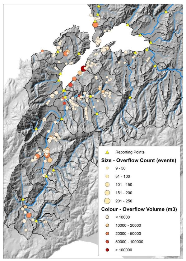
Figure 2.5: Wastewater overflow locations
