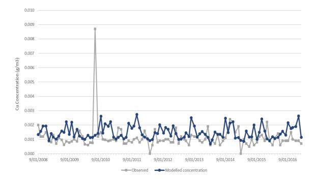
Figure A.18: Comparison of monthly Dissolved Copper concentration at Porirua at Glenside
