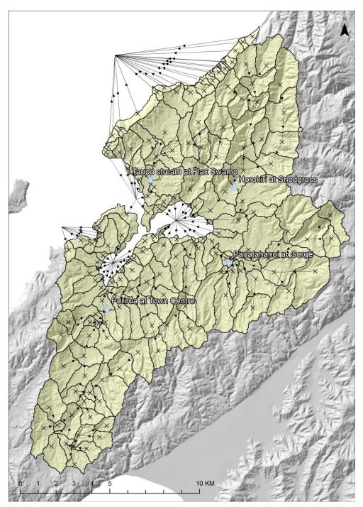
Figure 2.2: Sub-catchment boundaries, node-link network, and flow calibration sites
