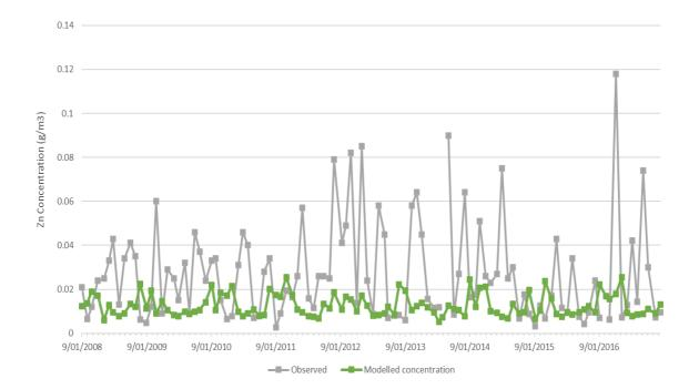
Figure A.15: Comparison of monthly Dissolved Zinc concentration at Porirua at Milk Depot. – Note: two extreme values are not displayed (0.25 g/m<sup>3</sup> on 7/08/2012, 0.33 g/m<sup>3</sup> on 16/02/16)
