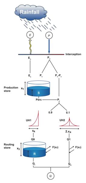
Figure 3.1: GR4J Rainfall-Runoff schematic (eWater, 2015)
