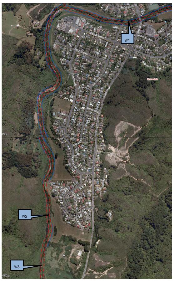
**Figure 3-2:** View of Wainuiomata application area (lower reach) showing design channel (red dash) and buffer zone (blue dash) and monitoring sites W1, W2 and W3 (from Cameron, 2015)
