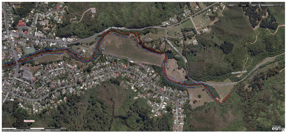
Figure 3-1: View of Wainuiomata application area (upper reach) showing design channel (red dash) and buffer zone (blue dash)
